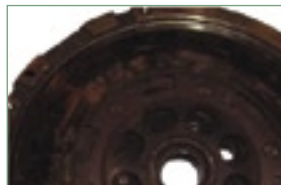
Fig.2 Image of the DMF illustrating the metal dust generated from wear to the flywheel casting
