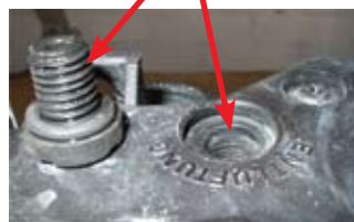
Image 2 Bleed screw fully removed to aid air bleed
