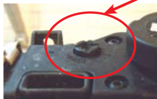
Image 1 Bleed screw located next to the Filler cap
