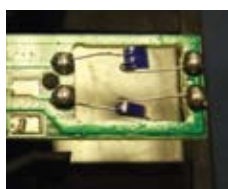
Image 3 Chinese element showing corrosion
