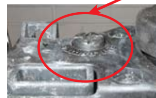
Image 3 Bleed screw partially removed
