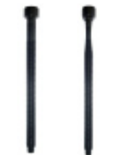
Image 2 A new Head Bolt A stretched Head Bolt
