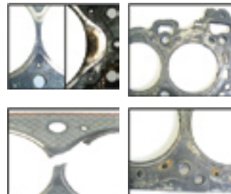
Image 3 - Four details of failed head gaskets as a result of reused bolts
