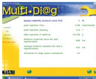
Multi-Diag's Actia connected to a Peugeot DPF system
